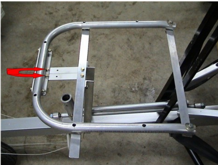
These bolt heads clear the seat.
